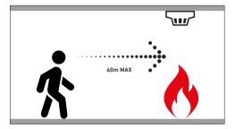
A person searching a zone for a fire in a non-addressable fire system should not have to travel more than 60m to identify the source of a fire.
