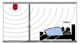
For areas where people are sleeping, sounder devices should produce a minimum 75dB(A) at the bed-head with all doors shut. In buildings providing sleeping accommodation for deaf or people with impaired hearing, bedrooms should have both audible and visual alarms. (Note: Visual Alarm Devices are not intended to wake sleeping persons).
