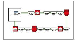
Short circuit isolators limit the effect of one fault to 2000m<sup>2</sup> and to a single storey of the building. '2 simultaneous faults on a circuit should not disable protection within an area greater than 10.000m<sup>2</sup>.
