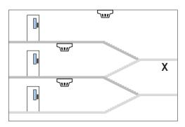
Enclosed stairways should have a detector at the top of the stairway and on each main landing.
