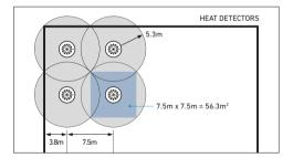
When mounted on a flat ceiling, heat detection devices have an individual coverage of 5.3 m radius. However these radii must overlap to ensure there are no 'blind spots'. Therefore individual coverage can be represented by a square measuring  $7.5 \text{m} \times 7.5 \text{m}$  giving an actual area coverage of  $56.3 \text{m}^2$  per device.
