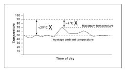
The minimum static response to heat devices should not be less than  $29^{\circ}\text{C}$  above the average ambient temperature, or less than  $4^{\circ}\text{C}$  above the highest temperature the device can expect to experience.
