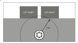
Vertical shafts like lifts and open stairways should have a device mounted within 1.5m of any opening. (This is not necessary for enclosed stairways, because as noted below, there are detectors on every landing within the stairway).
