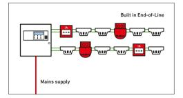
Fire resistant cabling is now required within the whole fire alarm system including the mains supply cables. The use of non-fire resisting cables whether mechanically protected by fire-resisting construction or not, will no longer comply with BS 5839-1.
