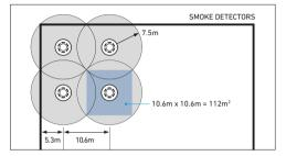
When mounted on a flat ceiling, smoke detection devices have an individual coverage of 7.5m radius. However these radii must overlap to ensure there are no 'blind spots'. Therefore individual coverage can be represented by a square measuring  $10.6m \times 10.6m$  giving an actual area coverage of  $112m^2$  per device.
