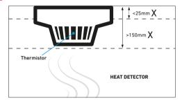
The sensing element of a heat detection device should not be less than 25mm below ceiling, and not greater than 150mm below ceiling.
