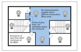
The minimum sound level should be 65dB(A) or 5dB(A) above a background noise which is louder than 60dB(A) (if lasting more than 30 seconds) and at a frequency of between 500Hz and 1000Hz. The maximum sound level should not be greater than 120dB(A) at any normally accessible point. May be reduced to 60dB(A) in stairways, enclosures up to 60m² and specific points of limited extent.
