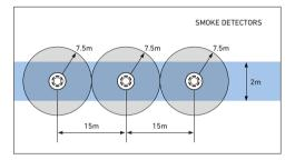
In corridors less than 2m wide the horizontal spacing of detectors may be increased, the areas of coverage need not overlap as in the case of a room. Any corridor over 2m wide is deemed a room and device spacing should follow the standard for rooms (see page 9).
